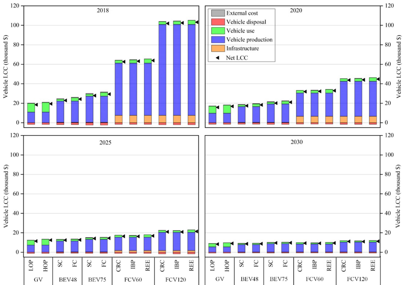
Fig. 7 Lifecycle cost comparison of different types of vehicle models in different scenarios. Note: x-axis represents the five vehicle models in different scenarios; Net LCC=infrastructure construction cost + vehicle production cost + vehicle use cost – vehicle disposal cost + external cost.
